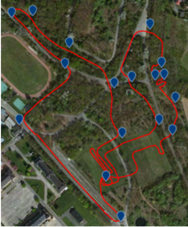
Figure 5.7: Digitized version of the cyclocross course of the Rectavit Series Leuven (2020). Red line is the GeoJSON course linestring. The blue markers are GeoJSON point features and are representing the cameras and their respective identifiers (camera id), which are hidden in this picture.
