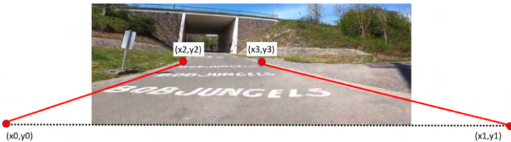
Figure 4.3: Example of Bob Jungels' name painted on the "La Redoute" climb. The coordinates for the homography are also annotated on the image. The coordinates are roughly representing the road boundaries.
