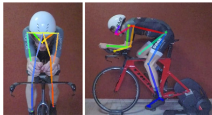
Figure 3.3: Rider skeleton detection (lab set-up)
