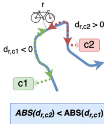
Figure 5.9: Illustration of closest camera along the course principle. Rider r is “snapped” on the blue course line following the direction of the arrow. Cameras c1 and c2 are also projected on the course linestring. Distance d is the distance from rider r to a camera c with a given index, following the course path. Negative distances are cameras behind the rider, positive distances are cameras the rider is approaching. Closest camera is the camera with the smallest absolute distance.
