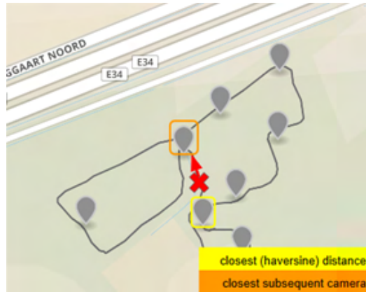
Figure 5.8: Camera setup on a test course. The red X is the current location of the rider following the course in the direction of the red arrow. Yellow circled marker is the absolute closest camera. Orange circled marker is the next camera the rider will visit on the course.
