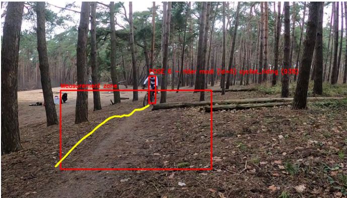
Figure 3.12: Illustration of the ROI principle on a video frame of a cyclocross training session. The red rectangle is the region of interest. Results of pose detection, tracking and post processing are illustrated by the yellow path within the ROI.
